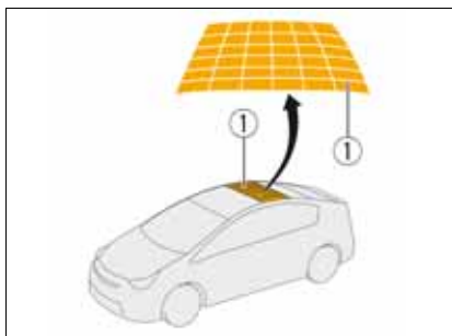
① Painel solar
